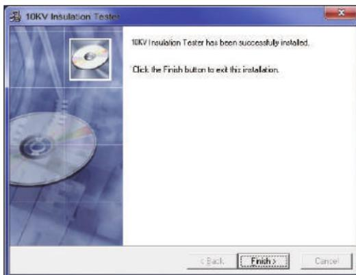
(Note: If your personal computer system is Windows 7, it will indicate the driver automatically. It's necessary to install the driver if your computer system is not windows 7, then the driver is in the compact disk (CD). The directory is " E:USB DRIVER/CDM 2.08.24 WHQL Certified x 86-32 bit".)
