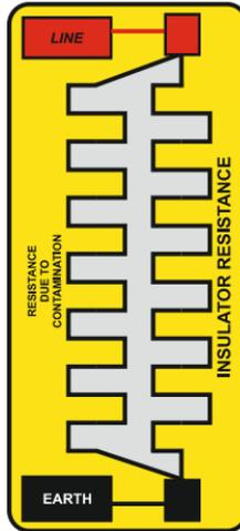
RESISTANCE DUE TO CONTAMINATION CAN BE VERY LOW AND LOWER THE TOTAL RESISTANCE.
