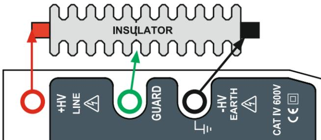
2. Switch ⑪ the function rotary switch to turn on power and select test voltage from 1kV, 2.5kV, 5kV or 10kV respectively.
