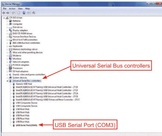
(Note: USB Serial Port will indicate different “COM” automatically)
